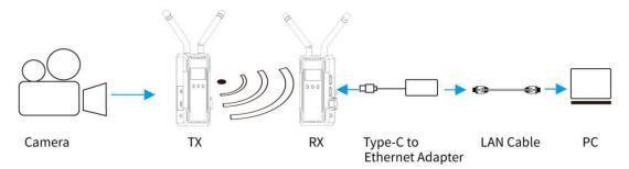
2. As the picture shown above, connect the Type-C to Ethernet adapter with computer via LAN cable.
