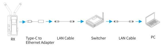
Connect a monitor to the receiver. Then connect the receiver to the router via the Type-C to Ethernet adapter. If the blue light flashes on the adapter, it indicates that the connection is good. The monitor will show the IP address on the left bottom.
