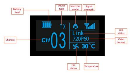
1) Channel switch: press" $\triangle$ "or" $\nabla$ "to change channels. Press" $\Box$ "to confirm the channel.
